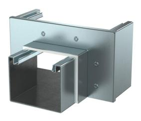
Reducer with intumescent fire protection mesh for symmetrical reduction of straight duct sections from PLM D 1220 to PLM D 0810. Suitable for direct wall and ceiling mounting, mounting below system floors and on support systems. Tool-free joint mounting with PLM SI joint connector. The cover is snapped on without tools, allowing rapid inspection and retroassignment. The cover overhang allows offset cover mounting for continuous equipotential bonding of the entire duct section.
