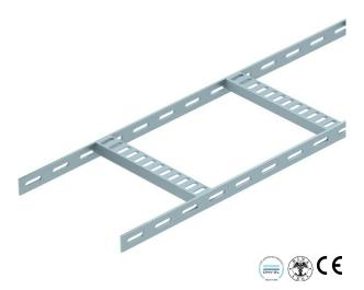
Shipbuilding cable ladder with perforated side rail of side height 25 mm with welded, perforated trapezoidal rungs which open in a downwards direction. Load tested according to IEC in conjunction with connector, type SLV. The shipbuilding cable ladder, including fittings, is also available in stainless steel on request. Powder coating according to RAL colours possible.
